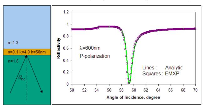
The above example simulates the surface plasmon excitation using Kretschmann-Raether method. The SPR is produced at the interface between the metal (n=0.1 k=4.0) and the dielectric (n=1.3) using a p-polarized planewave at the angle of incidence of about 59.3 degree.
