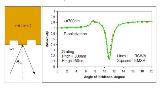
In this example the reflectivity as a function of incident angle obtained by EMXP compares well with that obtained Rigorous Coupled Wave Analysis (RCWA).
